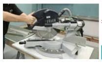
Cut the edging profile using the chop saw.
