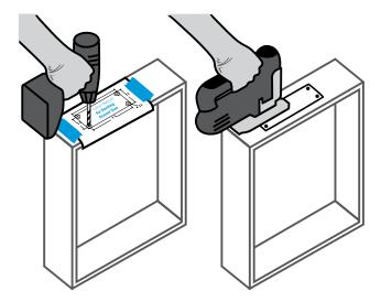
**Step 5** - Reinstall the drawer box and slide the Docking Drawer Duo or Trio receptacle box through the cutout. Secure it with the 4 wood screws provided.
