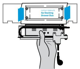
**Step 4** - With a 1/2" drill bit, drill a hole in each corner, being careful not to splinter the wood on the inside of the drawer box. Using one of the 1/2" holes, insert a jigsaw and then make the required cutouts in the drawer box.
