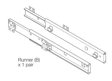
Using the runner drilling pattern shown in diagram 1, fix the runner (B) and required additional 2 mm spacers (D) using 16 x 4.5 x 30 mm pan head screws (C) to the internal side of the carcase with the bottom runner fixing point a minimum of 10 mm up from the floor level of the cabinet.
