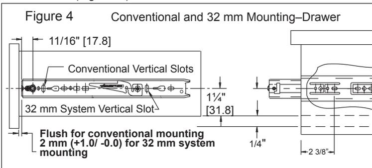
1. Make sure the ball bearing retainers in the cabinet side are fully forward. Install drawer into cabinet. Close the drawer.
