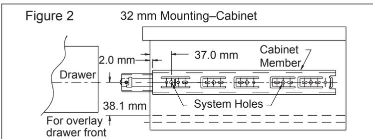
2. Use only the 32 mm system holes or the wood screw holes located at the tip of the breathing tabs. Do not use any other holes on the cabinet member for mounting (Figure 3).
